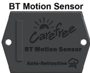
The optional BT Motion sensor detects awning motion caused by windy conditions. The system gauges the motion of the awning's front edge (roller tube or lead rail). When the motion exceeds the preset threshold, the system retracts the awning.
