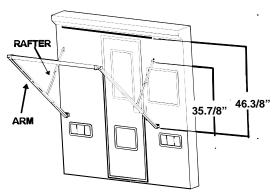
**C.** Position the bottom bracket of the arms so that the previously made marks line up with the center line of the bottom bracket bolt.
