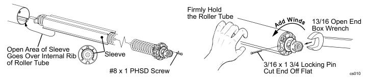
**NOTE:** It will be necessary to firmly support and brace the roller tube. A second person is required to hold the roller tube.
