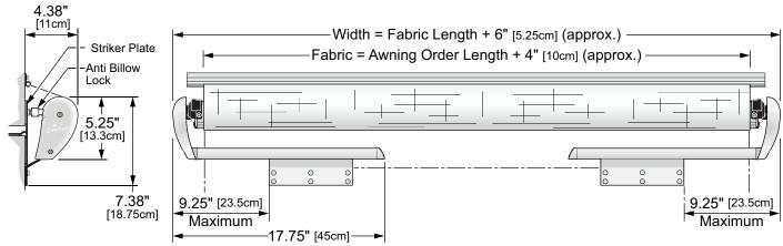
Shown with tall bracket, dimensions are approximate. Actual dimensions may vary based on installation and room configuration.
