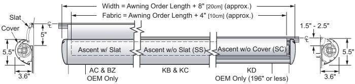
Dimensions are given for reference only and may vary based on the slide-out configuration and installation specifics. For detailed installation information, refer to the product manuals available on-line at www.carefreeofcolorado.com
