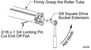
8. Hold the pin in place and slowly release the ratchet handle. When there is no pressure on the handle, remove the square drive from the spindle. Press the pin in as far as possible then place tape over the head of the pin to avoid the pin coming out.
