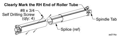
3. Attach the left tube half to the splice using four (4) #8 x 3/4 self-drilling screws. Match the screw pattern in the right roller tube half.
