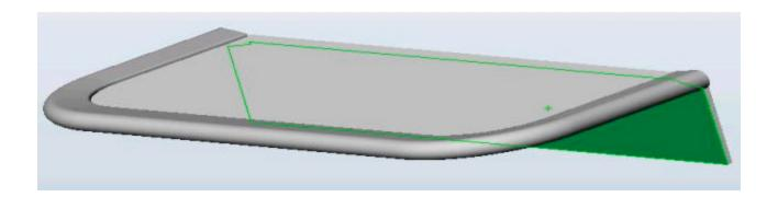
If replacing the canopy on an Omega awning that utilizes a wind deflector, install the supplied trim strip along the edge of the wind deflector as show. This will prevent the fabric from tearing as it overlaps the sharp edge of the deflector.
