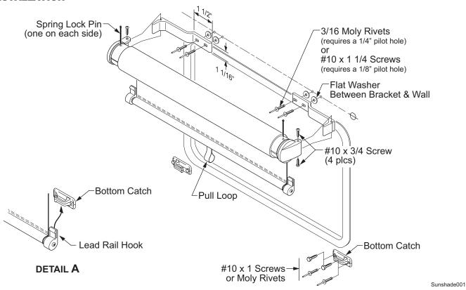
1. Lift the shade up and center over the window. The mounting brackets should be positioned just above the window frame.
