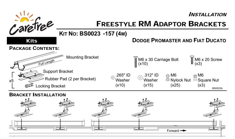
NOTE: To correctly support the awning, the locking brackets and support brackets must be arranged as shown. BS0023c
