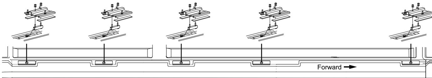
**NOTE:** To correctly support the awning, the locking brackets and support brackets must be arranged as shown. BS0023c
