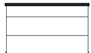
HS Configuration Canopy construction with horizontal seams
