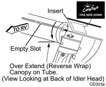
*Tip: Clean the slot and lightly spray the inside with a dry silicone lubricant. This will aid with sliding the canopy in.*
