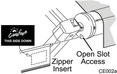
5. Slide the polyrod edge of the insert into the open slot of the roller tube. Orient the insert with the seams toward the vehicle.
