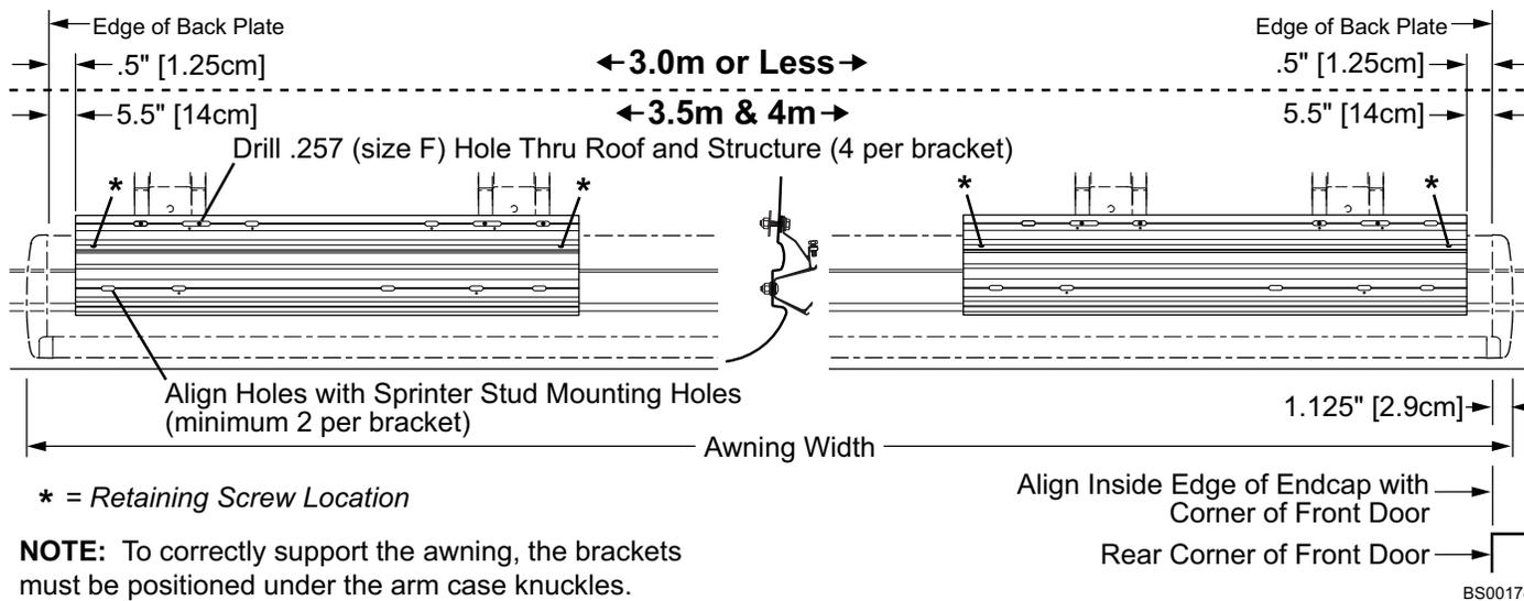
**NOTE:** To correctly support the awning, the brackets must be positioned under the arm case knuckles.
