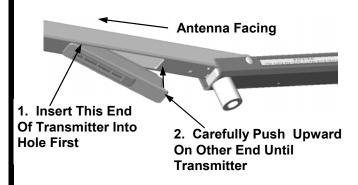
NOTE: ANTENNA, WIRES AND SWITCH NOT SHOWN FOR CLARITY
