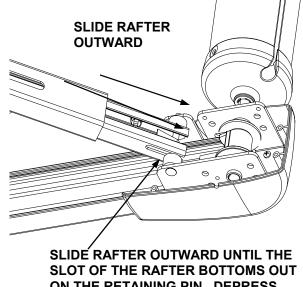
ON THE RETAINING PIN. DEPRESS SPRING AND REMOVE RAFTER
