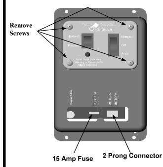
Step Three: Install the Power Control Module and Power Control Switch (cont.)
