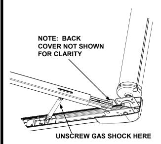
C. Remove top bracket lag bolts that are attaching the top bracket to the vehicle. Take care not to scratch the vehicle with the top brackets when removing.
