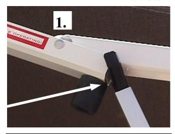
STEP 3: TO OBTAIN PROPER TENSION ON THE WIND BRACE IT MAY BE NECESSARY TO ADJUST THE BRACE BY PUSHING INWARD ON THE SPRING BUTTON AND LOCATING IT IN A DIFFERENT HOLE, EITHER DECREASING OR INCREASING THE OVERALL LENGTH OF THE BRACE. (SEE LOWER LEFT) PROPER ADJUSTMENT IS WHEN THE SPRING IS AT LEAST SLIGHTLY COMPRESSED WHEN THE BRACE IS IN THE POSITION AS SHOWN DIRECTLY BELOW.
