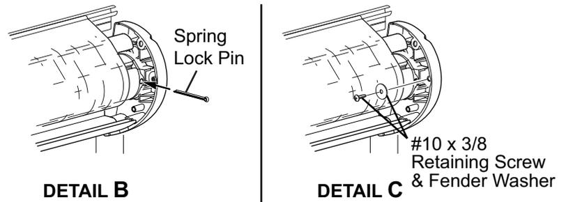
**IMPORTANT NOTE:** The XL model has two springs. A second spring locking pin must also be inserted through the LH spindle and taped in place before continuing.
