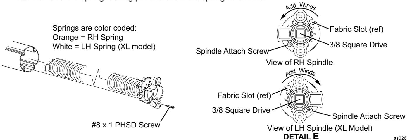
2. After the spring is unwound, remove the #8 x 1 pan head square drive screw that attaches the spindle assembly to the roller tube and save.
